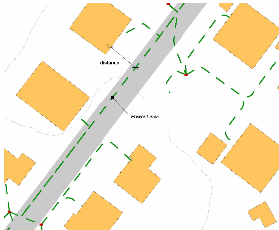
Figure 1: Distance from construction to power line
